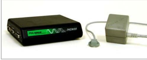
The PATRIOT sensors are not only easily embedded, but due to the true 6DOF the PATRIOT delivers, the SEP system can track both position and orientation of laparoscopic instruments. The tracked position and orientation data is used as input to real-time 3D simulation of surgical techniques and procedures.
