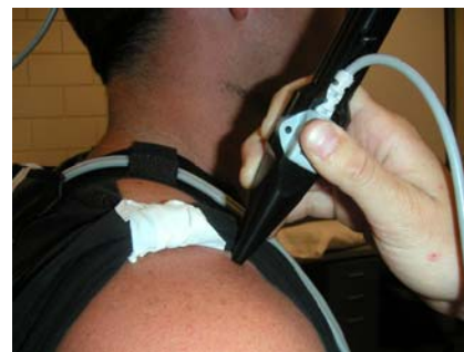
Figure 2. Magnetic pen used to locate anatomical landmarks.
