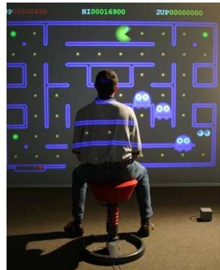
In an area surrounding the center the mapping is linear; thereafter, the distance is mapped as linear plus a cubic factor. This allows the user to travel at higher speeds by tilting the seat further in the direction of travel.
