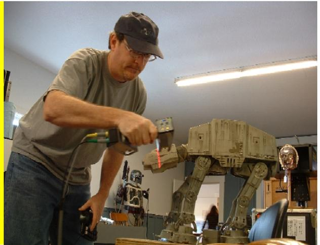
The FastSCAN Cobra is a lightweight, handheld laser scanner, which you sweep over an object – just like spray painting. This lets you scan those hard to reach places other scanners cannot, as Steve reported from the set of Star Wars III in Sydney: *"in fact we have never been able to scan rubber prosthetic masks effectively in the past because of undercutting fill-in from our head scanner."*
