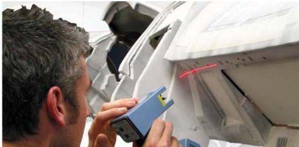
Technical expertise for the scanning process was supplied by ARANZ Scanning Limited. All metal components from the dash were removed and the dash was sprayed with a contrast-enhancing agent to give the black dash a more scanable surface. ARANZ scanned the whole dash at a resolution of around 0.5 mm. Post processing with FastSCAN created a high-resolution water-
