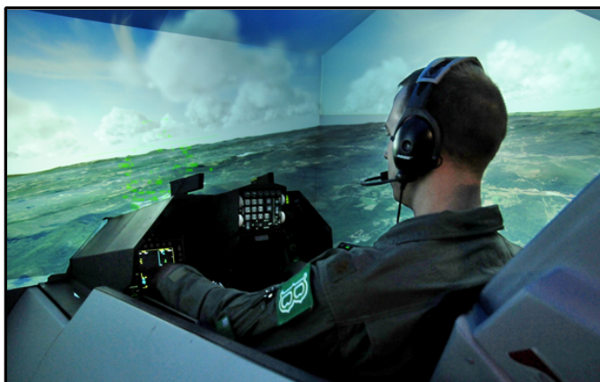
Figure 1: One of four cockpit simulators at the new F-16 MTC, located at the ANG base at the Burlington International Airport, Burlington, VT. The multi-channel synchronized view, driven by VRSG, is rendering the VT virtual terrain built by MetaVR. Photo courtesy of MetaVR; photo credit to SSgt. Dan DiPietro, 158 FW, Vermont Air National Guard.
