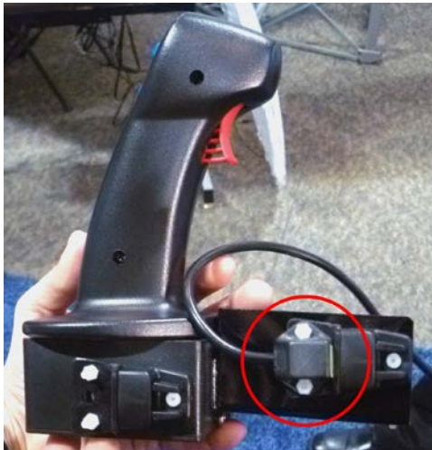
Polhemus 6DOF Sensor attached to gun manipulator
